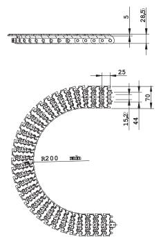
A plastic chain with a friction surface. Recommended surrounding temperature is -18 - +50 °C. Recommended maximum work load at 20° is 100 kp/1000N.
