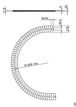
A plastic chain with a friction surface. Recommended surrounding temperature is -18 - +50 °C. Recommended maximum work load at 20° is 200 kp/2000N.
